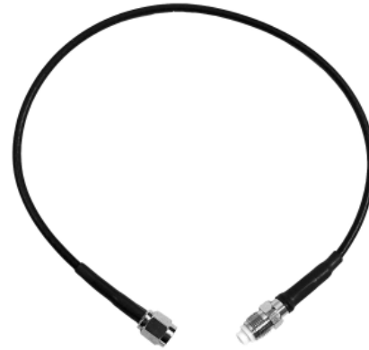
FME Female to RP - SMA Female Jumper (12 in RG174 Coax)
